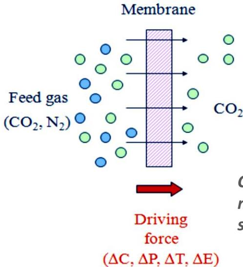
The driving force for CO<sub>2</sub> permeation can be a difference in concentration (ΔC), pressure (ΔP), temperature (ΔT) and electric potential (ΔE) of CO<sub>2</sub> and N<sub>2</sub> at either side of the membrane.
